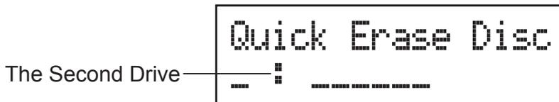
5. When the erase job is in process, you should see the O and o are blinking by turns.
