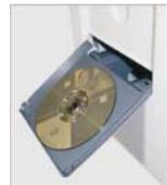
When the Reject Disc Tray is open as shown, rejected discs will be sent to this tray. The tray will hold up to three discs. Once the tray is full, the overflow discs will be pushed off the tray. The use of a container is suggested to collect the overflow discs.
