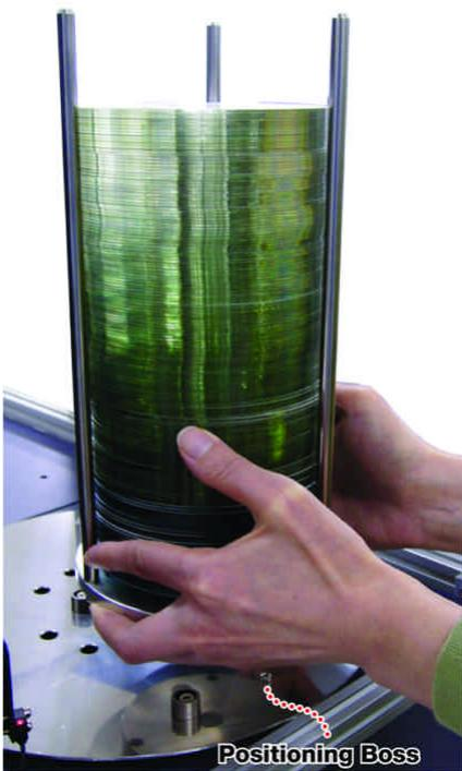
After placing the magazine on the turntable, pat the sides of the disc stack so that it stands vertically. Also take care not to allow the disc stack to be slanted.
