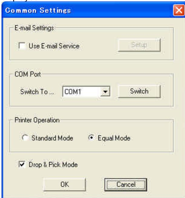
In this window, users setup the e-mail service feature that will send an e-mail to the specified mail address to notify completion of a job and error occurrence, select the COM port that is used by the PC to communicate with the TRILOGY main unit, specify how to use inkjet printers (Standard/Equal), and activate/deactivate Drop&Pick mode. These items will not be changed frequently. Please note that print related errors in the printers will not be notified via e-mail.
