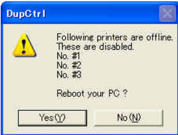
Confirm that the USB cables between the printers, hub, and PC are connected properly. If a cable is disconnected, re-connect it and click on [Yes] to reboot the PC. The TRILOGY starts the PC reboot process.
