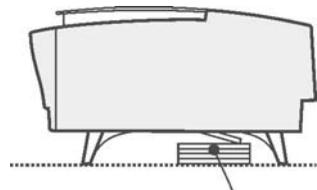
Rejected discs come out beneath the unit
