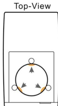
JuniBox processes discs in a First In, First Out (FIFO) sequence. During a duplication session, if a disc refill is required, before the loader becomes empty, gently load additional discs.
