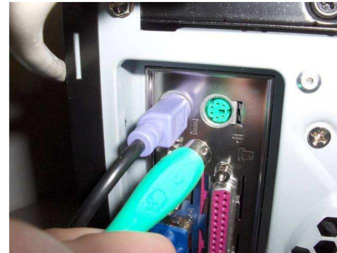
Connect the power, keyboard, mouse, and monitor cables to the color-matched ports.
