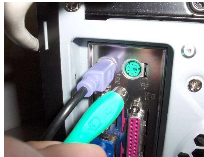
Connect the power, keyboard, mouse, and monitor cables to the color-matched ports.
