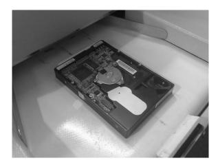
For the second pass, the hard disk drive should be rotated through 90 degrees. Keeping the PCB side facing upwards, and the drive should be placed against one of the conveyor belt guides to prevent the drive moving during the degauss process.
