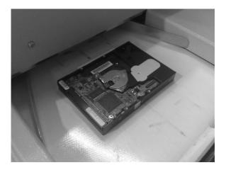
During prolonged continuous operation the unit will eventually overheat. At this stage a red warning indicator on the front panel will illuminate before returning to the standby mode when cooled. Approximately 20 minutes should be allowed before attempting any further erasures.
