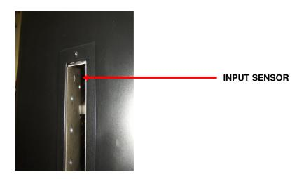
The sensor is recessed 5mm (0.2") so a small brush will be required to clean it. A tooth brush is an ideal for this purpose. Press the brush over the hole so some of the bristles go through the hole shown above and clean the sensor. The other half of the sensor is on the side of the chute directly opposite the one shown in the Photograph above and should be cleaned in the same way.
