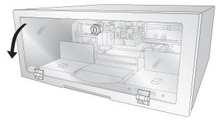
• The Publisher will automatically position the cartridge carrier and Robotic Disc Transporter to the center position allowing for easy access to the bins.
