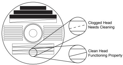
If the Yellow, Magenta, Cyan or Black diagonal lines printed on the disc show breaks, repeat the cleaning procedure. If nozzles still appear to be clogged, remove the cartridge and gently wipe the nozzle area sideways with a clean water-dampened cloth. If after several cleanings a color still does not appear on the test print, the cartridge may be damaged or empty and may need to be replaced.
