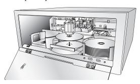
4. The Recorder Tray then automatically shuts. Robotic Disc Transporter will automatically check the Input Bin to make certain that only one disc was picked.
