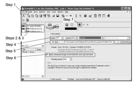
Note: It is possible to use the drive in the duplicator for the Recorder drive and the reader/source drive. This is recommended to reduce recording variables which are introduced by using different drive models for reading and recording.
