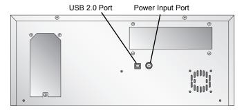
The USB 2.0 Interface is connected to an open USB 2.0 port on your PC with the USB 2.0 cable, included with your Publisher.
