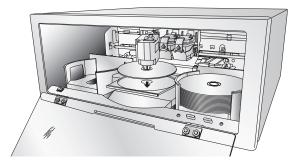
8. Print time varies according to which print mode has been selected (section 3-A). In most cases, print time takes no more than 2 minutes. After printing the first disc, the Publisher's Printer Disc Tray opens automatically. The Robotic Disc Transporter moves the finished disc to the Output Bin.
