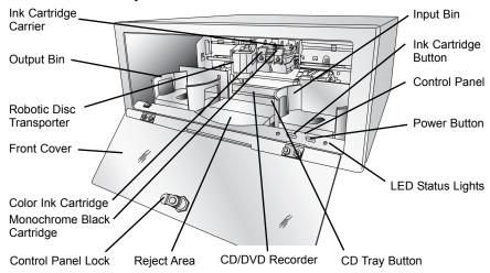
The **Robotic Disc Transporter** moves discs from the Input Bin, to a CD/DVD Recorder, to the printer, and finally to the Output Bin.
