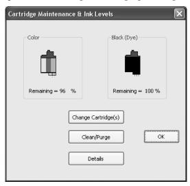
Select **Clean** button to send a simple test pattern to the printer. Be sure to have a disc in the Bravo's input bin and the front cover closed. The test pattern, shown below, purges ink through nozzles of your ink cartridge to clear any blockages. The test pattern will show if the nozzles require any further cleaning.
