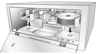
• Load the Input Bin (the bin located on the right-hand side of the Publisher) with 25 blank discs and place the bins on the mounting pegs.
