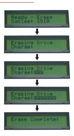
**Note:** After degaussing, hard drives should not be not be reused as they are stressed in the erasure process. Some backup tapes may not be reusable after degaussing due to the servo track being erased.
