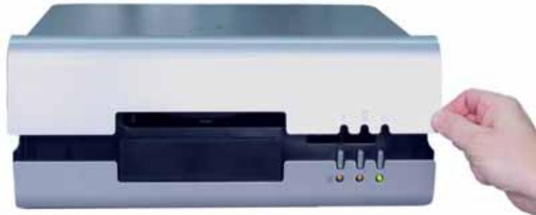
2. Lift the ink cartridge latch to the open position.
