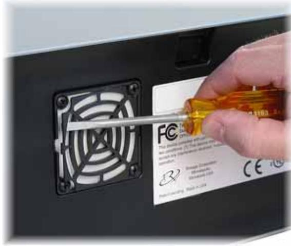
2. Gently pull the fan filter housing away from the back of the Rimage 480i.
