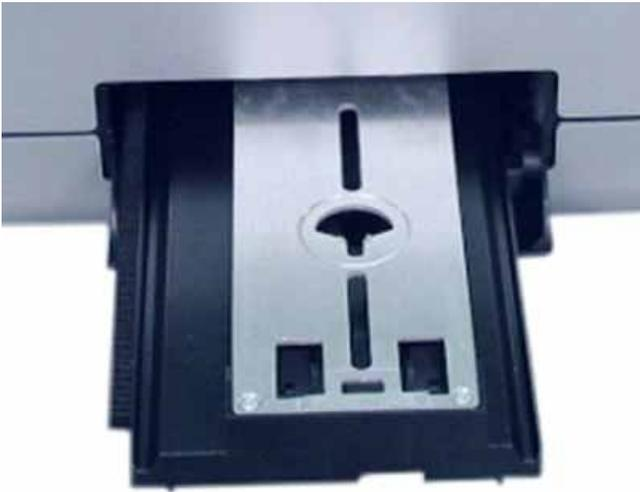
2. Carefully place the disc on the printer tray, aligning the hole in the disc with the small pins on the printer tray.
