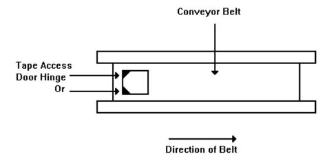
DVC Pro cartridges must be passed through the degausser a second time having turned the cartridge over.
