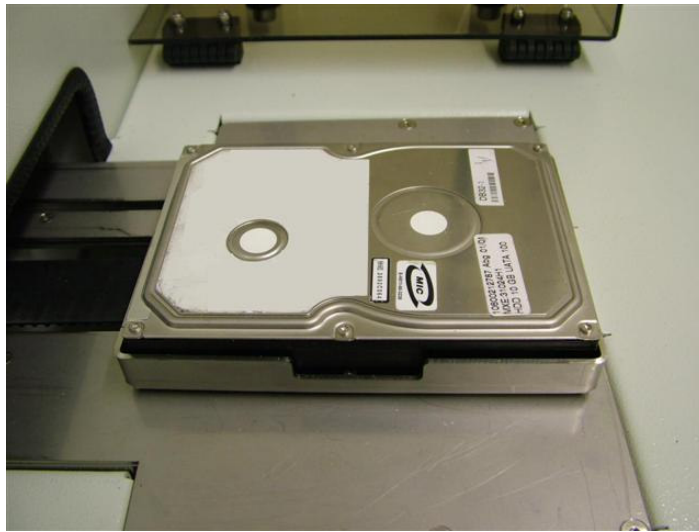
HDD inserted into caddy ready for erasure
