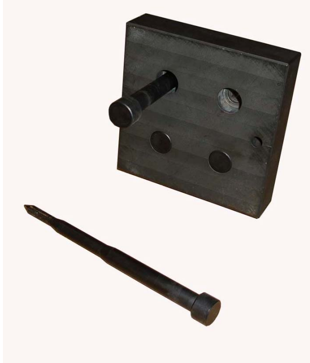
Figure 9: Destroyer Spike removed from Destroyer plate
