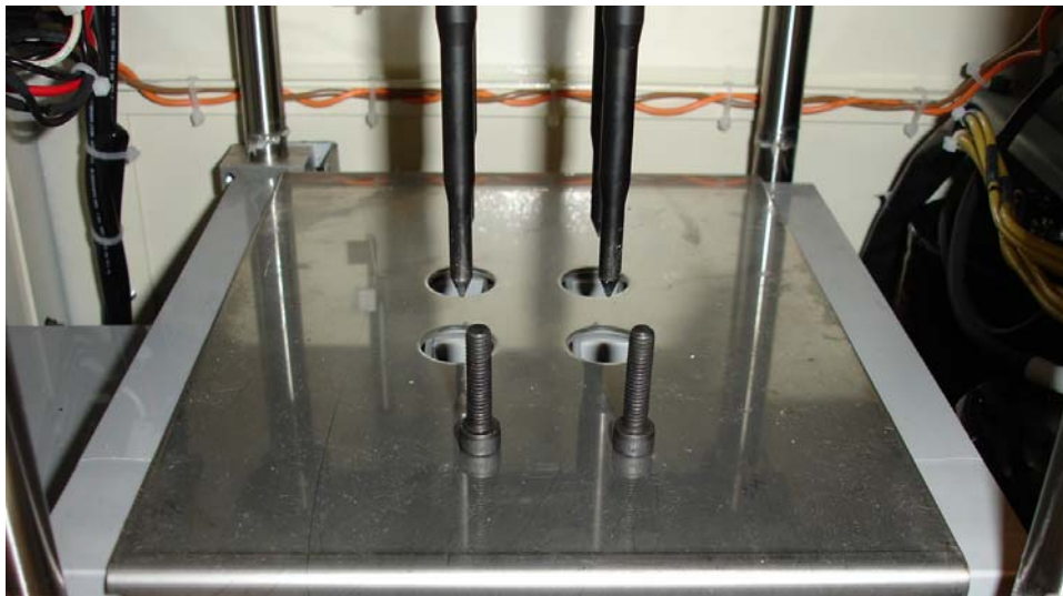
Figure 6: Both bolts removed
