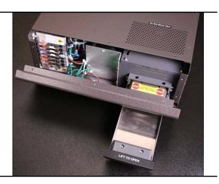
To change the jumper position, pull the brown jumper wire from terminal on the right side of the fuse block and move it to the corresponding terminal that matches the power mains outlet voltage.
