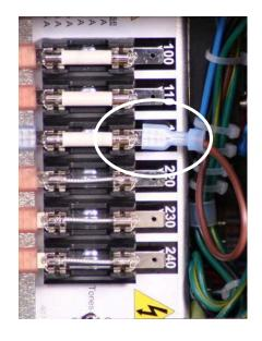
Notice, this photo shows the correct jumper setting for 240 VAC.
