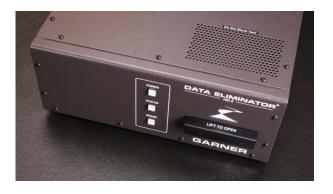
Open the drawer and tilt back the front panel as shown.
