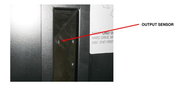
The sensor is recessed 5mm (0.2") so a small brush will be required to clean it. A tooth brush is an ideal for this purpose. Press the brush over the hole so some of the bristles go through the hole shown above and clean the sensor. The other half of the sensor is on the side of the chute directly opposite the one shown in the Photograph above and should be cleaned in the same way.
