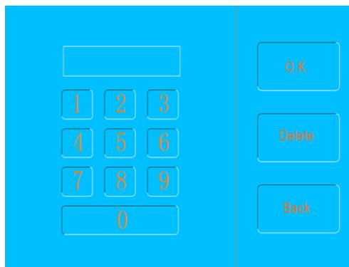
The screen displays: Password Field、 O.K.、 Delete、 Back. Enter the password of system in password field (default code: **1111**) and press“O.K.”to confirm. Press “Delete” to clear . Press “Back” to back to the main menu.
