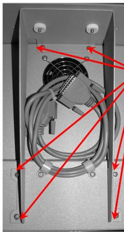
Fix bracket to CopyDisc with 6 screws
